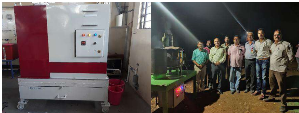
Plate No. 5.2 Pyrolysis fuel equipment – Plasto Green
