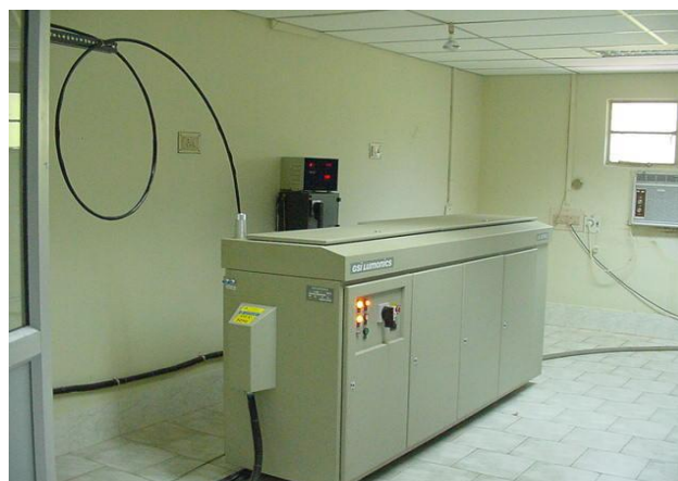
Figure.1. Solid state Nd:YAG Laser source at WRI used for experimental work [18].
