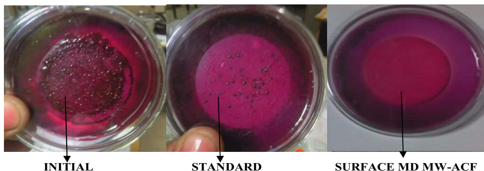
Figure1- comparison of Standard and surface modified MW-ACF colonies obtained on M-Endo Agar
