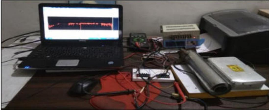
**Figure-1. Experimental setup of air ion counter.**
