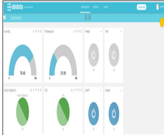
Figure-3. A control dashboard for a remote user using cloud server to control and monitor home Appliances.
