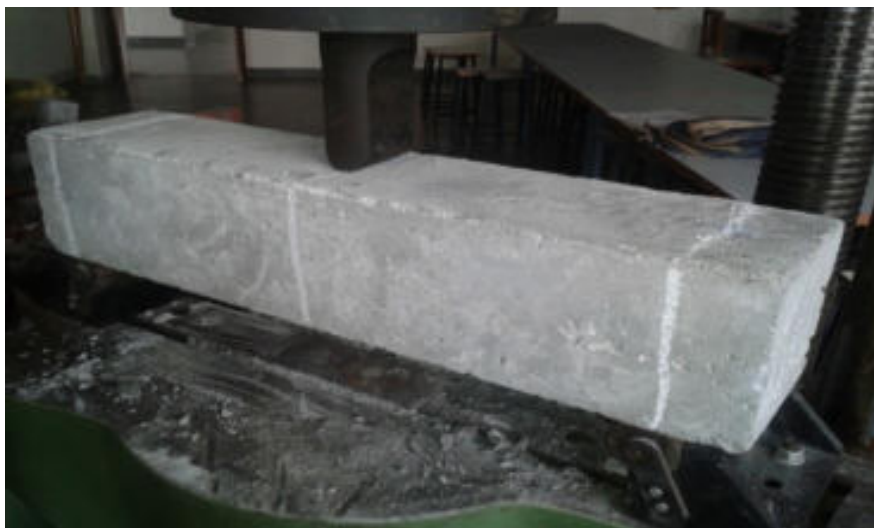
Figure-7. Flexural strength of beam specimen.
