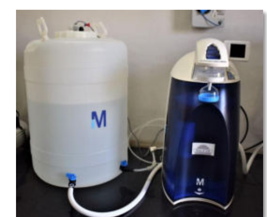
Ultra pure Water Purification System
